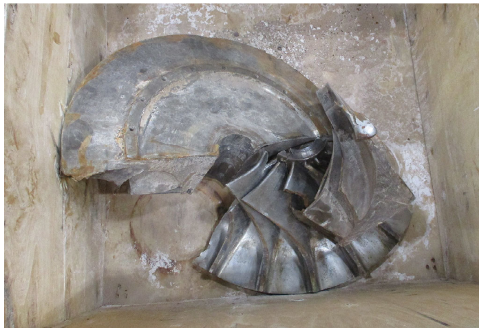
Figure 1: The inlet nozzle, casing, and impeller were all damaged beyond repair.
