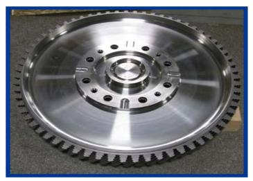
Replacement of both disks was required because their useful life limit was reached. Often, however, using remaining life analysis techniques pioneered by RMS personnel, we are able to extend the useful life of power turbine disks beyond their rated operating lives, which is typically 100,000 hours. RMS has been able to certify disks for operation up to 200,000 hours.
