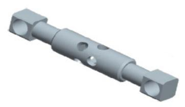
ring should be expanded from its relaxed shape to allow easy bolting of the retaining ring segments to the diaphragm. RMS used state-of-the-art 3D modeling software to design a spreader tool that will be used to aid in future assemblies and disassemblies of the ring. The design of the tool was based on a turn-buckle that will be bolted to the existing holes in the shear ring and used to either expand the ring during assembly or shrink the ring during disassembly.
