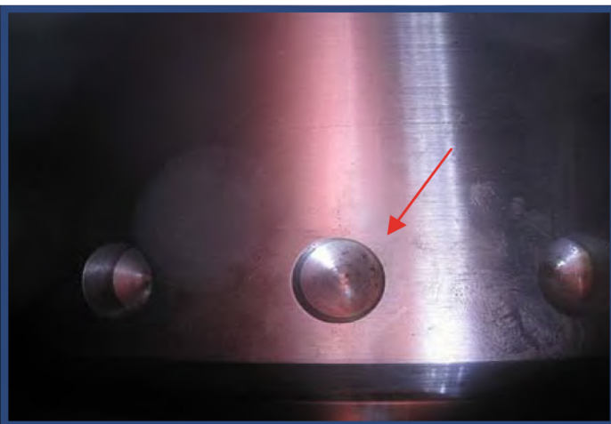
Figure 2: The red arrow points to the expander speed probe targets. Note the expander targets are more widely spaced than the turbine targets.
