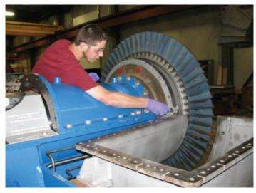
rebladed disc. The rotor rebuild and refurbishment of the bearing and seal assembly, along with a rebuild of the exhaust casing to add stiffeners to eliminate casing cracking during operation were completed at the RMS manufacturing facility. In addition, a new coupling guard was fabricated and machined. Field service was provided to reassemble the expander and rework the intermediate casing and exhaust transition piece. RMS completed the entire scope within the customer's turnaround schedule.
