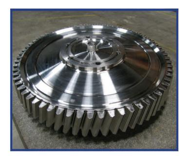
RMS recently shipped two large super alloy power turbine disks to separate gas pipeline customers. These disks replaced Ingersoll-Rand and Dresser-Clark components that had exceeded their useful operating lives. (Note that, prior to replacing disks, RMS can perform a Remaining Life Analysis to determine whether replacement is truly necessary.) The approximately 40 inch, 1,600 pound forgings are among the largest super alloy disks used in turbomachinery.
