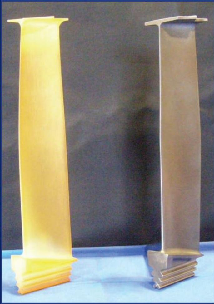
RMS was recently awarded a contract by a major domestic utility to provide spare FT4 Rotor Blades. Combining the use of traditional inspection techniques such as height gages, micrometers, and calipers, RMS incorporated the newest reverse engineering methods such as high accuracy laser scanners, 3D modeling software, FEA analysis software, and prototype modeling creation whenever possible.
