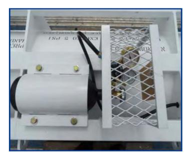
Due to the many advantages, rotors are frequently stored in fabricated steel canisters. These containers provide significant protection during either shipping or storage. They are also constructed to enable the container to be stowed vertically. As a result, the risk of rotor bowing is prevented that would otherwise occur during long-term horizontal storage. In the horizontal position, the rotor would sag and detrimentally affect API level rotor balance.
