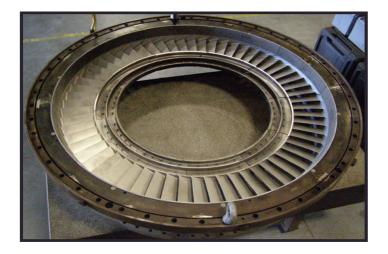
inventory of used spares, along with parts from the currently operating turbine, were inspected to determine the most suitable components for repair.
