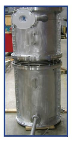
RMS was contracted to replace the coupling guard between an expander and motor on a PRT train. The typical coupling guard design accommodates axial growth through a sliding fit sealed with "O" rings. This design has been prone to oil leaks due to poor installation.
