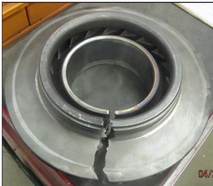
Figure 1: Failed Centrifugal Compressor Impeller due to Surge Event
