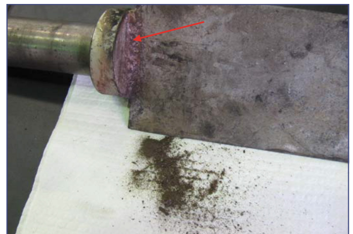
Figure 3: The arrow points to pulverized screen material that was centrifuged by the rotor and deposited on the stationary surfaces including variable guide
