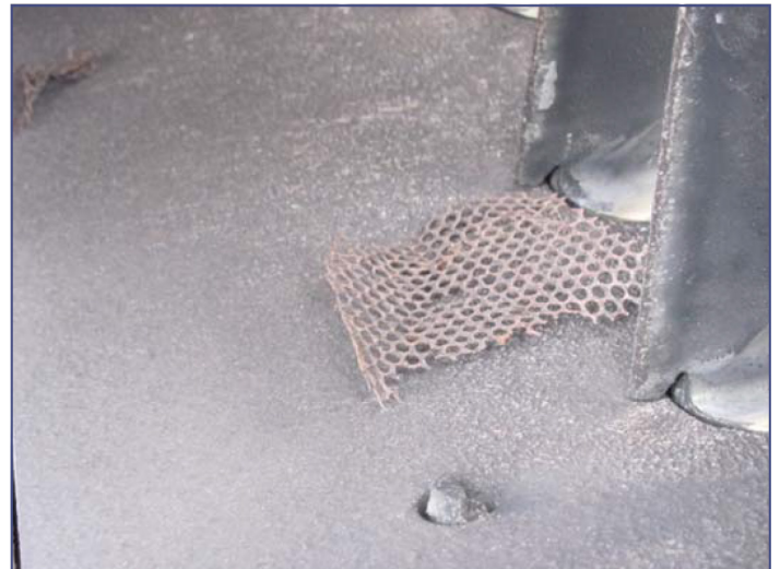
Figure 2: A section of inlet silencer screen was found near the inlet guide vanes.
