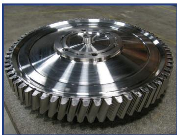
RMS recently shipped two large super alloy power turbine disks to separate gas pipeline customers. These disks replaced Ingersoll-Rand and Dresser-Clark components that had exceeded their useful operating lives. (Note that, prior to replacing disks, RMS can perform a Remaining Life Analysis to determine whether replacement is truly necessary.) The approximately 40 inch, 1,600 pound forgings are among the largest super alloy disks used in turbomachinery.
