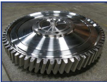
RMS recently shipped two large super alloy power turbine disks to separate gas pipeline customers. These disks replaced Ingersoll-Rand and Dresser-Clark components that had exceeded their useful operating lives. (Note that, prior to replacing disks, RMS can perform a Remaining Life Analysis to determine whether replacement is truly necessary.) The approximately 40 inch, 1,600 pound forgings are among the largest super alloy disks used in turbomachinery.
