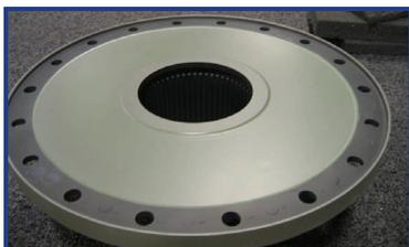
RMS has provided a direct replacement for a P&W model FT4 free turbine coupling. The coupling was manufactured from an ultrasonic quality forging. The original output shaft geometry was duplicated and the original coupling design retained, thereby maintaining overhung weight and torsional stiffness identical to the original configuration. The coupling was subjected to RMS quality standards throughout manufacture.
