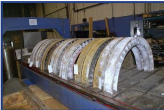
A major steel supplier contracted with RMS to provide an overhaul of an axial compressor rotor and flowpath components. After RMS performs visual, dimensional and NDT inspections of the compressor components to evaluate usability, the rotor will be polished, rebladed, balanced and prepped for long term storage. The flowpath variable stators and fixed stators will be weld repaired and upgraded per RMS standards for return to service.
