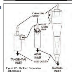
Figure #2 - Cyclonic Separation Technologies
