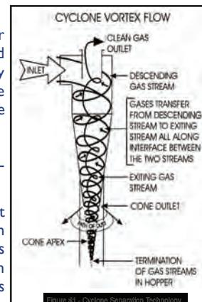
Figure #1 - Cyclone Separation Technology
