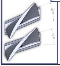
Furthermore, since RMS has been using a FARO laser scanner to scan all axial compressor rotor blades that pass through the shop, RMS now has the capability to take orders for new rotor blades for any inspected rotor, even after it has left the building. Through continued adoption and implementation of cutting-edge technology, RMS is constantly increasing its capabilities, helping us deliver the best products and services possible to our customers.
