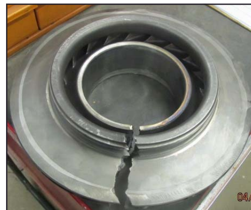
Failed Centrifugal Compressor Impeller due to Surge Event
