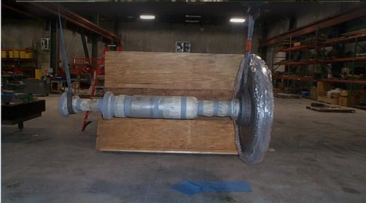
**PROBLEM:** Emergency turnaround inspection & repair of IR JP125 power turbine rotor
