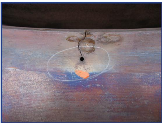
Flange Cracking Around Expansion Pin
