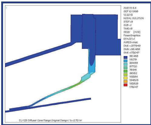
Original Design Showing Extreme Stresses in the Area Where Cracking Occurred
