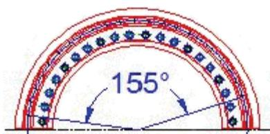
Partial arcs are most commonly used in the first, or control, stage and extraction stage nozzles. However, they can be found throughout all stages of a turbine.
