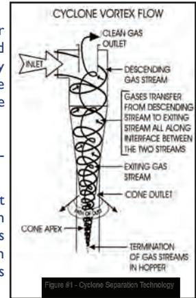
Figure #1 - Cyclone Separation Technology
