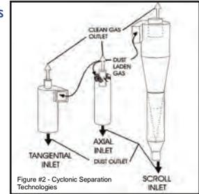
Figure #2 - Cyclonic Separation Technologies
