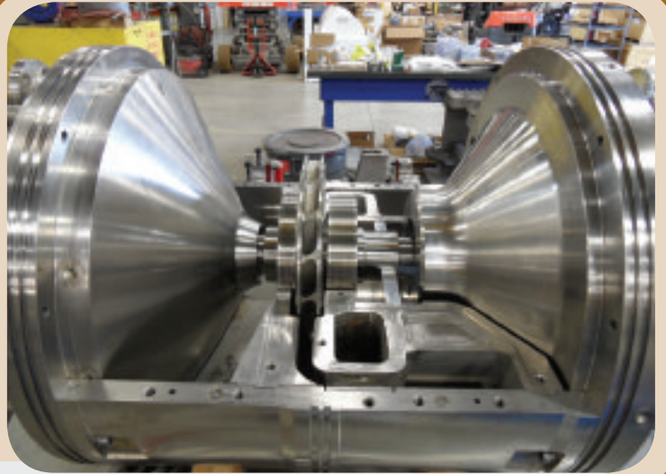
■ RMS refurbishes and upgrades process (left) and pipeline centrifugal compressors including new custom-engineered aerodynamic assemblies (right).
