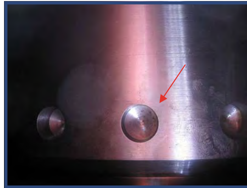
Figure 2 - The red arrow points to the expander speed probe targets. Note the expander targets are more widely spaced than the turbine targets.
