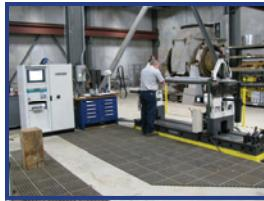
In order to evaluate the distortion of large gas casings, we have developed the capabilities to perform run out inspections. Our milling machine has been a real asset and quite a few small machine jobs have been processed on it with good results.
