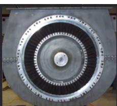
RMS developed a procedure that would allow for an obsolete, 20 year old expander exhaust casing and bearing support to be overhauled to provide a drop in spare exhaust casing and rotor, bearing & seal assembly (RBSA) for a unit that was installed in 2000.
