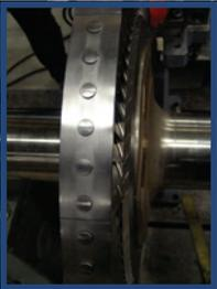
As part of the supply of a nitric acid plant air train, RMS has rerated and overhauled a customer's single stage GE expander from 2600 hp to 4700 hp. The work was accomplished within a 10 day window at a shop local to the Georgia plant.
