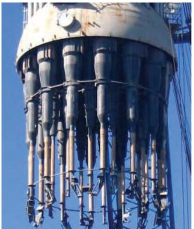
Figure #1 – FCC Regenerator Cyclones
