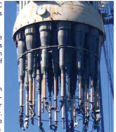
Figure #1 – FCC Regenerator Cyclones
