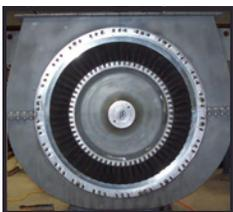
RMS developed a procedure that would allow for an obsolete, 20 year old expander exhaust casing and bearing support to be a overhauled to provide a drop in spare exhaust casing and rotor, bearing & seal ssembly (RBSA) for a unit that was installed in 2000.
