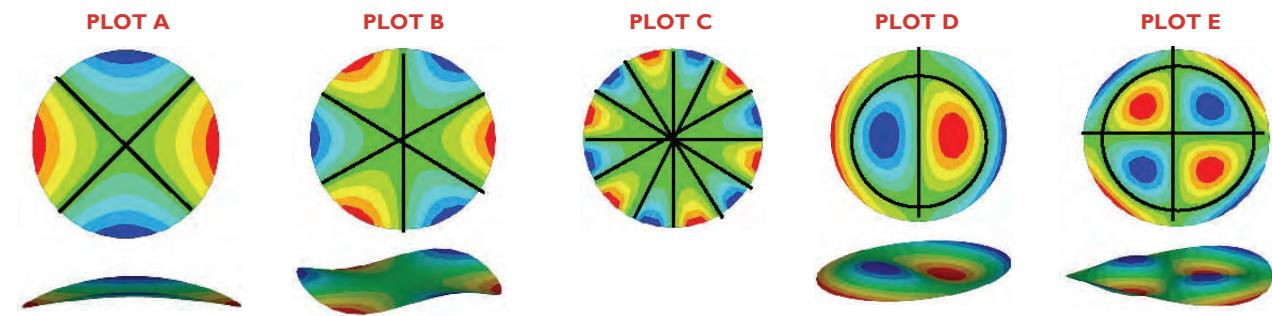
Plot E shows a two-nodal diameter, one-nodal circle flat plate mode. This is the potato chip mode shown in Plot A with a nodal circle.
