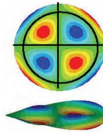
Plot E shows a two-nodal diameter, one-nodal circle flat plate mode. This is the potato chip mode shown in Plot A with a nodal circle.
