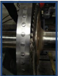
As part of the supply of a nitric acid plant air train, RMS has rerated and overhauled a customer's single stage GE expander from 2600 hp to 4700 hp. The work was accomplished within a 10 day window at a shop local to the Georgia plant.
