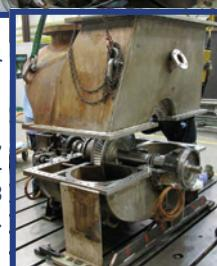
Overhaul and rerate services accomplished during the outage included disassembly, joint milling and line boring, casing hydrotest, bearing housing remachining and reassembly. The expander was installed on a new packaged baseplate with RMS's AXL508 11000 hp axial compressor and a rerated and refurbished Elliott QV7 steam turbine. The train was started in March of 2009 and is part of an acid plant expansion.
