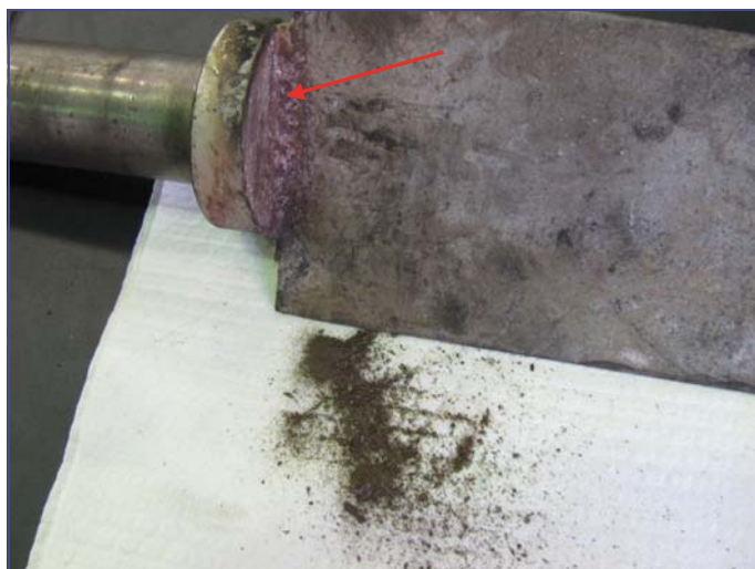
Figure 1 Note torn screen encapsulating the silencer material. The screen material was found at numerous locations in the flow path.
