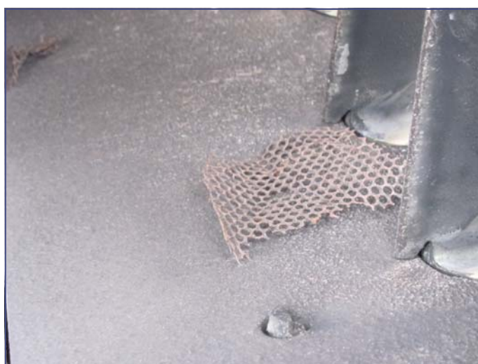
Figure 2 A section of inlet silencer screen was found near the inlet guide vanes.
