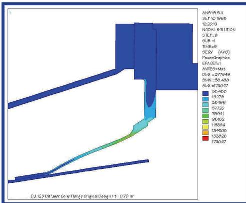
RMS's solution to the problem was to separate the hot flow-washed section of the annulus from the much cooler mounting flange. Axial expansion pins were employed to maintain concentricity of the duct. By doing so, thermal stresses were reduced to 20,000 psi. RMS provided three new Inlet Annuluses to our customer with the redesigned geometry. The design has been very successful, and completely eliminated the need for weld repair since the new ducts were placed in service.
