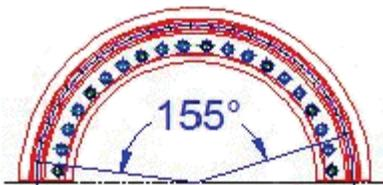
Partial arcs are most commonly used in the first, or control, stage and extraction stage nozzles. However, they can be found throughout all stages of a turbine.
