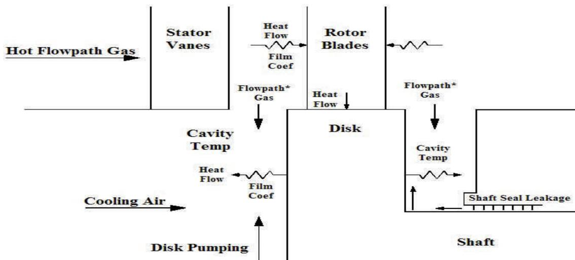
**\* Leakage from Flowpath (Disk Pumping - Cooling Air). If the Cooling Air Flow Rate exceeds the Disk Pumping Flow Rate then there is No Leakage from the Flowpath.**
