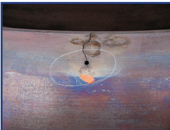
Flange Cracking Around Expansion Pin
